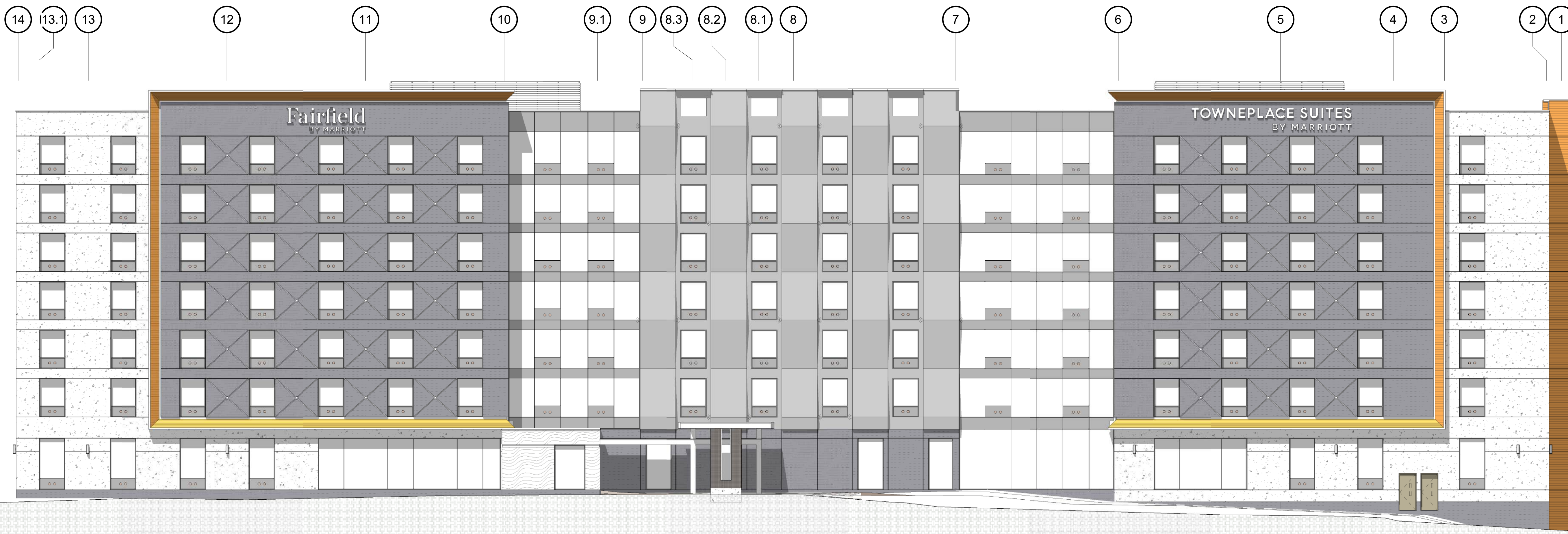
1 FRONT (NORTH) ELEVATION - COLOUR A303 3/32" = 1'-0"
