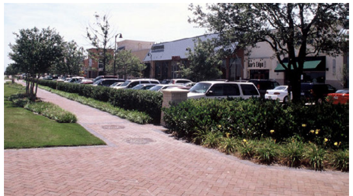
Lowered parking surfaces and landscaped buffers help screen parking areas from street view
