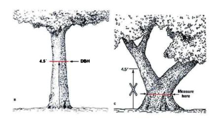
For a tree on a slope, measure up 1.4 meters along the axis of the trunk on both the high and low sides; DBH point is midway between these two planes.
