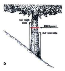
For a leaning tree, measure 1.4 meters along both the top and undersides of the trunk; DBH point is midway between these two planes.
