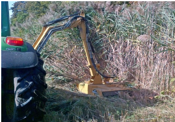
Boom mower cutting invasive Phragmites along a road
