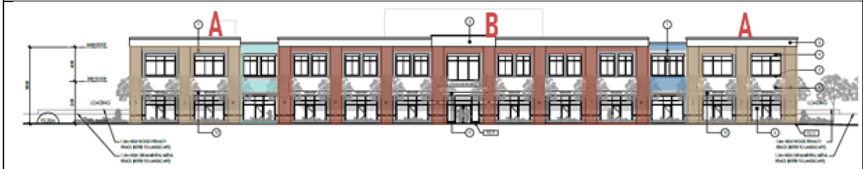
Figure 6.7 : Commercial East Elevation
