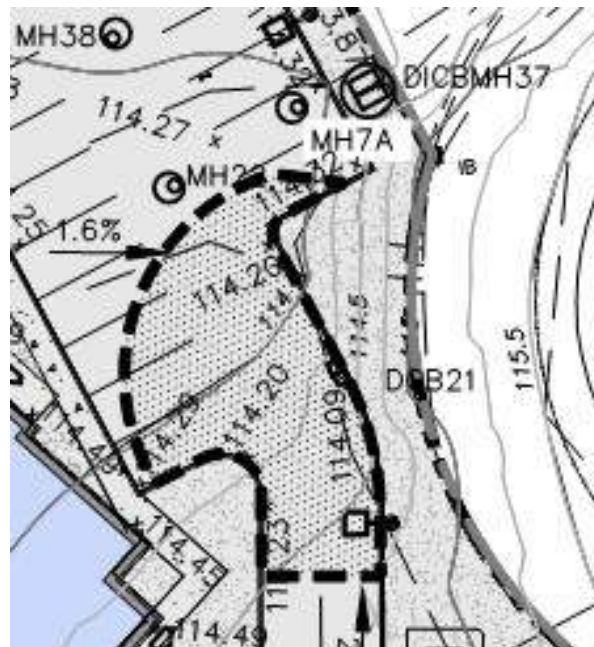
Figure 1 – Ponding in Subcatchment 202
