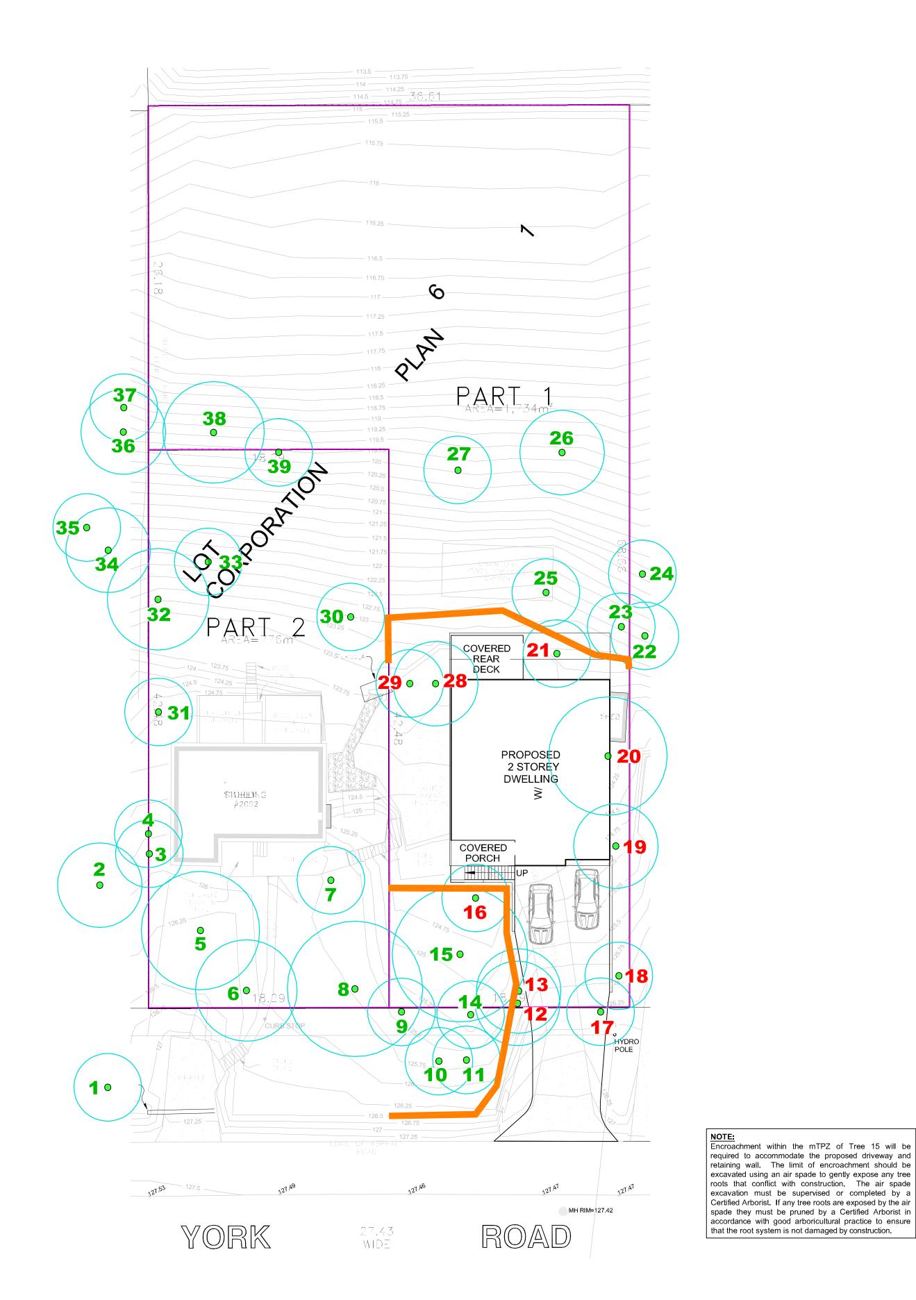
TREE PROTECTION NOTES: **FENCE DETAIL** 1.THIS DETAIL DOES NOT REPRESENT ANY PARTICULAR TREE **SPECIES** (Or at Distance Specified on the Tree Preservation Plan) 2. NO CONSTRUCTION **ACTIVITY. GRADE** CHANGE, SURFACE TREE PROTECTION TREATMENT, BARRIER TO CONSIST COMPACTION, **EXCAVATION OR ORANGE SNOW** STOCKPILING OF ANY **FENCE** KIND IS PERMITTED - PLACED ON METAL WITHIN THE T-BARS AT 3 METRE PROTECTED AREA. CENTRES. BARS TYP. 3000 mm MAXIMUM
