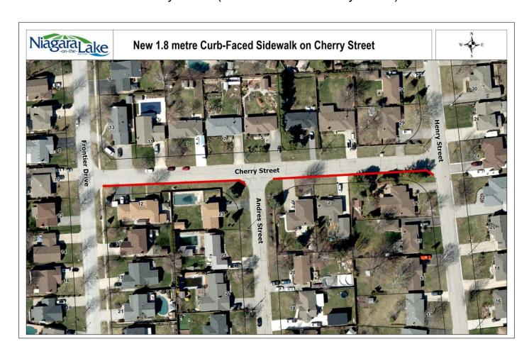
**WHAT:** The Town of Niagara-on-the-Lake, through its contractor Niagara Concrete Forming and Finishing, will commence with the construction of a new 1.8 metre curb-face sidewalk along the south side of Cherry Street, from Frontier Drive to Henry Street.
