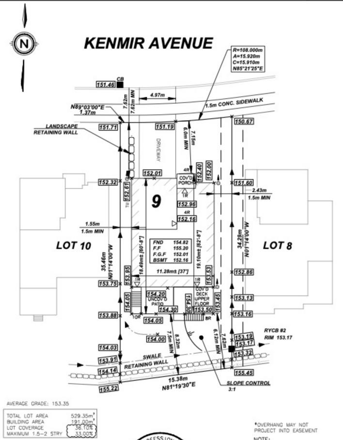
NOTE: THE MAXIMMUM HEIGHT OF THE CONCRETE SHOWING ON THE FOUNDATION WALL SHALL NOT BE MORE THAN 12" ABOVE THE FINAL APPROVED GRADE ELEVATION.
