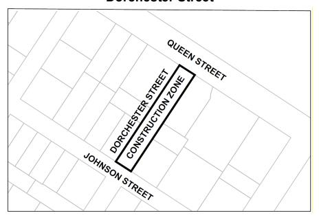
**WHAT:** The Town's contractor will be milling, making manhole adjustments, and conducting asphalt resurfacing on the following roads:
